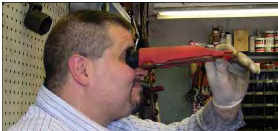
A refractometer is the most accurate way to check antifreeze concentration, which should be about a 50/50 mix with water for best performance.
