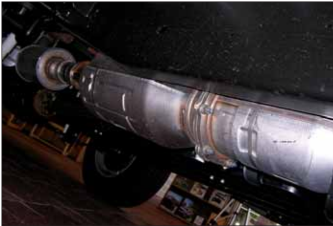
This photo shows the combined diesel oxidation catalyst, particulate filter and resonator that help to reduce emissions on a Ford 6.4L PowerStroke engine.
