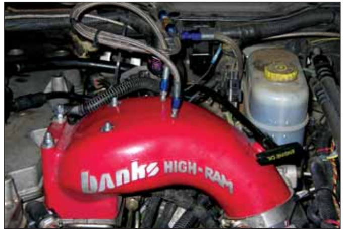
Installation of custom intake and exhaust systems will be problematic on 2007 and later diesels equipped with intake throttling, catalysts and particulate filters.
